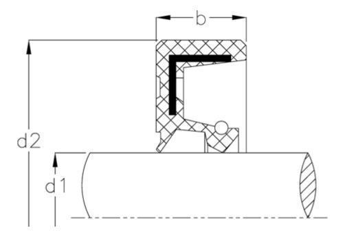
$\begin{array}{ll} b & = 8 \\ d1 & = 28 \\ d2 & = 48 \\ Material = NBR \end{array}$
